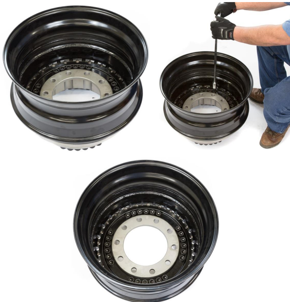
Tightening Inner Transducer Bolts with Torque Wrench and Torque multiplier (note: picture does not show mounted tire. Normal Install will have tire already mounted to Rim)
