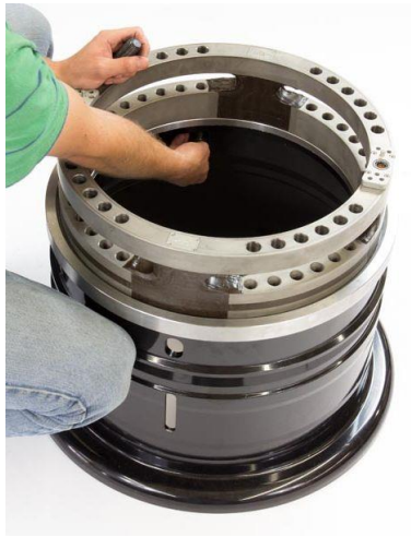
Wheel Force Transducer Mounted.
