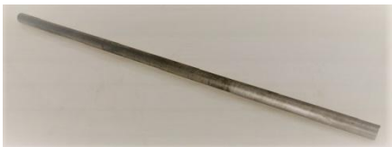
7. 0.500" low carbon steel rod; Cut to length, as needed.
