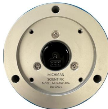
Figure 8: MUX to SR10AW/WFT Slip ring Adapter
