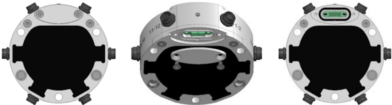
Figure 3: MUX bottom view showing connector cover removal.
